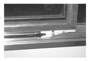
• Step 3: While keeping the screwdriver locked in this position and with panel still elevated, rotate the screwdriver approximately 1/4 of a turn so that the bottom of the guide rotates toward you.
