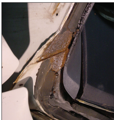
(Level 2-3 corrosion of pinchweld)
